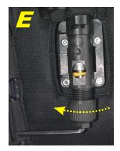
**E** Loosen the spring tension cap with the Allen key provided, turning it in the direction shown by the arrow, until the spring drops out of sight below the bottom of the release pin aperture of the trigger body.
