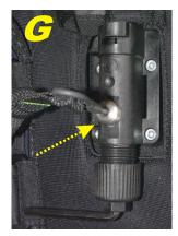
**G** Insert the release pin into the aperture, making sure it is fully pushed into the recess in the piston. Hold it in place with one hand and begin tightening the spring tension cap with the other hand.
