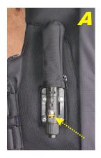
A This is how the trigger looks after activation. The release pin and lanyard have detached, the piston has slid towards the cartridge and the spring (marked with a yellow arrow) is visible.
