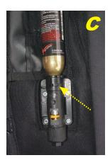
**C** When the retention lug on the bayonet fitting reaches the right hand side of the location slot (shown by the yellow arrow in the picture), you will feel the cartridge loosen in the trigger body.
