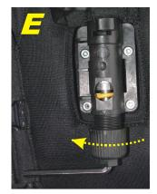
**E** Loosen the spring tension cap with the Allen key provided, turning it in the direction shown by the arrow, until the spring drops out of sight below the bottom of the release pin aperture of the trigger body.
