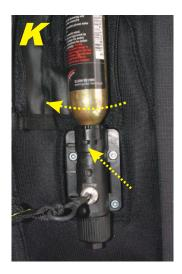
**K** Using light downward pressure, twist the CO<sub>2</sub> cartridge clockwise to the left, as shown by the direction of the top yellow arrow in the picture, until the location lug on the bayonet fitting is in the left side of the location slot.
