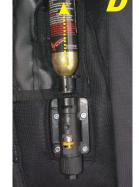
**D** Remove the empty CO<sub>2</sub> cartridge upwards away from the trigger body.
