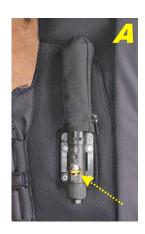
A This is how the trigger looks after activation. The release pin and lanyard have detached, the piston has slid towards the cartridge and the spring (marked with a yellow arrow) is visible.
